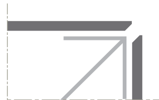
Figure 5: Mitred External Corner Detail
