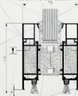
Door without a threshold - bottom cross-section
